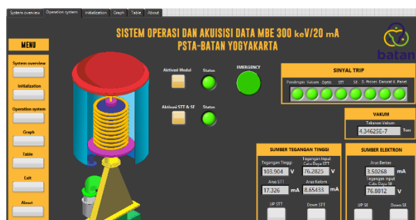
Figure 4. System HMI display MBE operation 300 keV/20 mA
