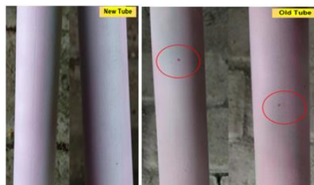
Figure 3. Penetrant test, surface of the new and old tube.
