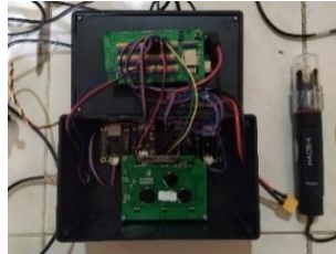
Figure 5 Installing a pH Sensor Device with Arduino Mega
