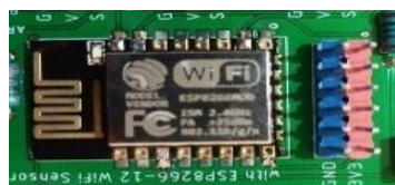
Figure 11 Installing an ESP8266 Module Device with arduino Mega
