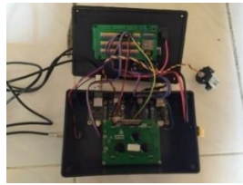
Figure 8 Installing a Turbidity Sensor Device with Arduino Mega
