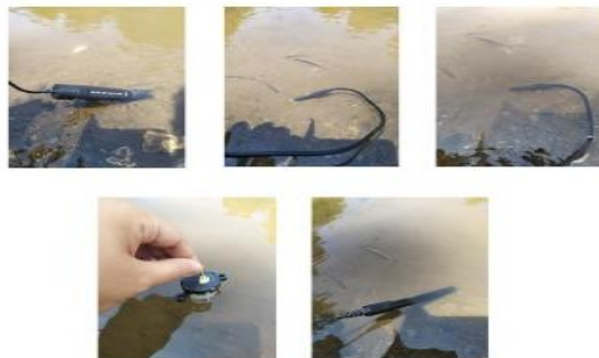
Figure 22 Overall pH, TDS, Temperature, Turbidity, and DO Sensors Detecting River Water
