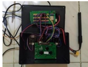
Figure 9 Installing a DO Sensor Device with Arduino Mega
